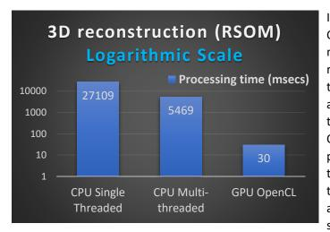
In RSOM (Raster Scan Optoacoustic Mesoscopy), the most demanding task is the 3D reconstruction process which can take minutes to complete. This is a big impediment for the usage of the device in medical applications. Optimization managed to achieve performance improvements in the range of **200 times faster t**han the multi-threaded CPU code and almost 1000 times faster than the single threaded CPU case. This
